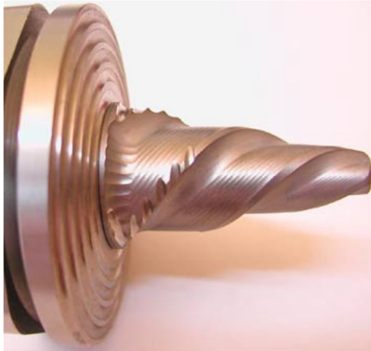
Figure 2-12: Tool for friction stir welding (SKB, 2010)
