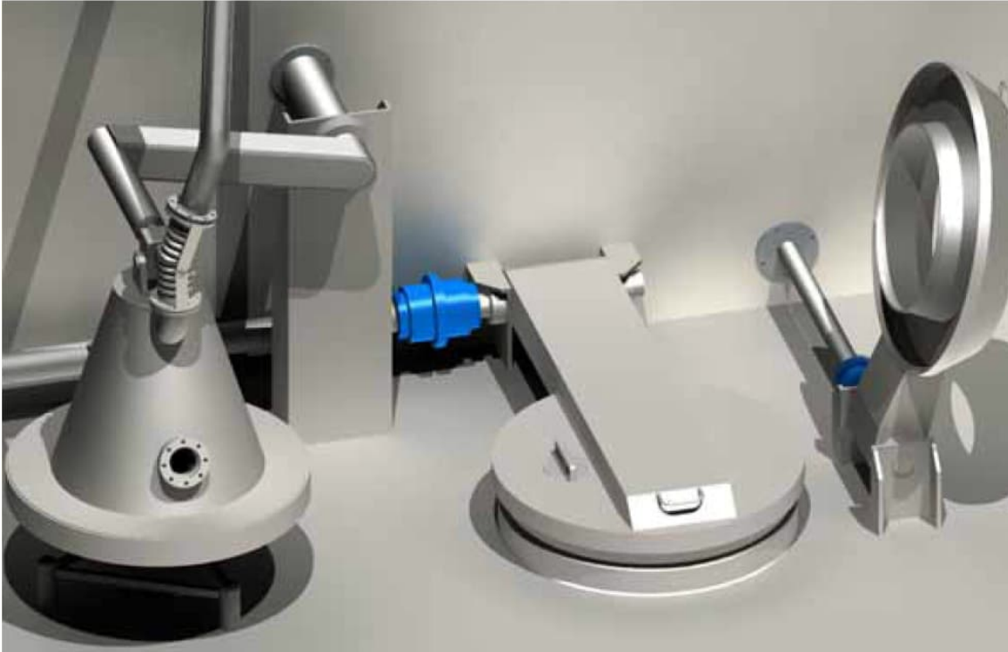
Figure 3-7: Equipment at the canister docking station: gas exchange cap on the left, covering hatch in the middle and protective cone on the right (Suikki 2006)
