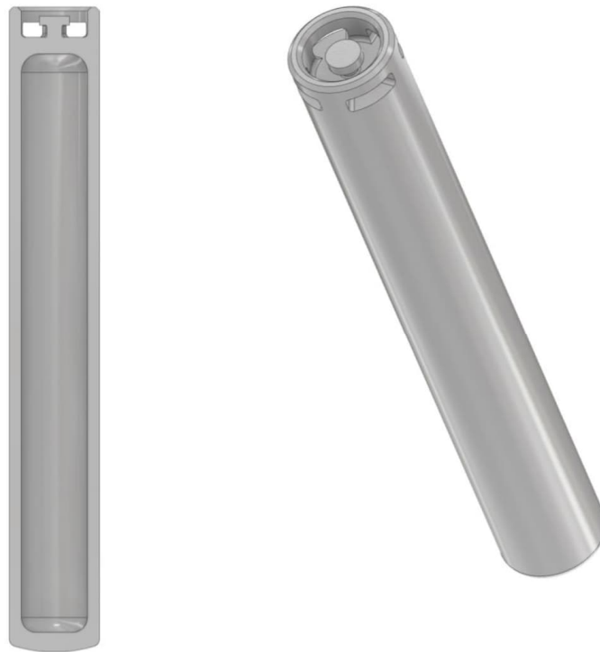
Figure 1-3: DBD-v1 canister for deep borehole disposal (Wunderlich et al. 2021).
