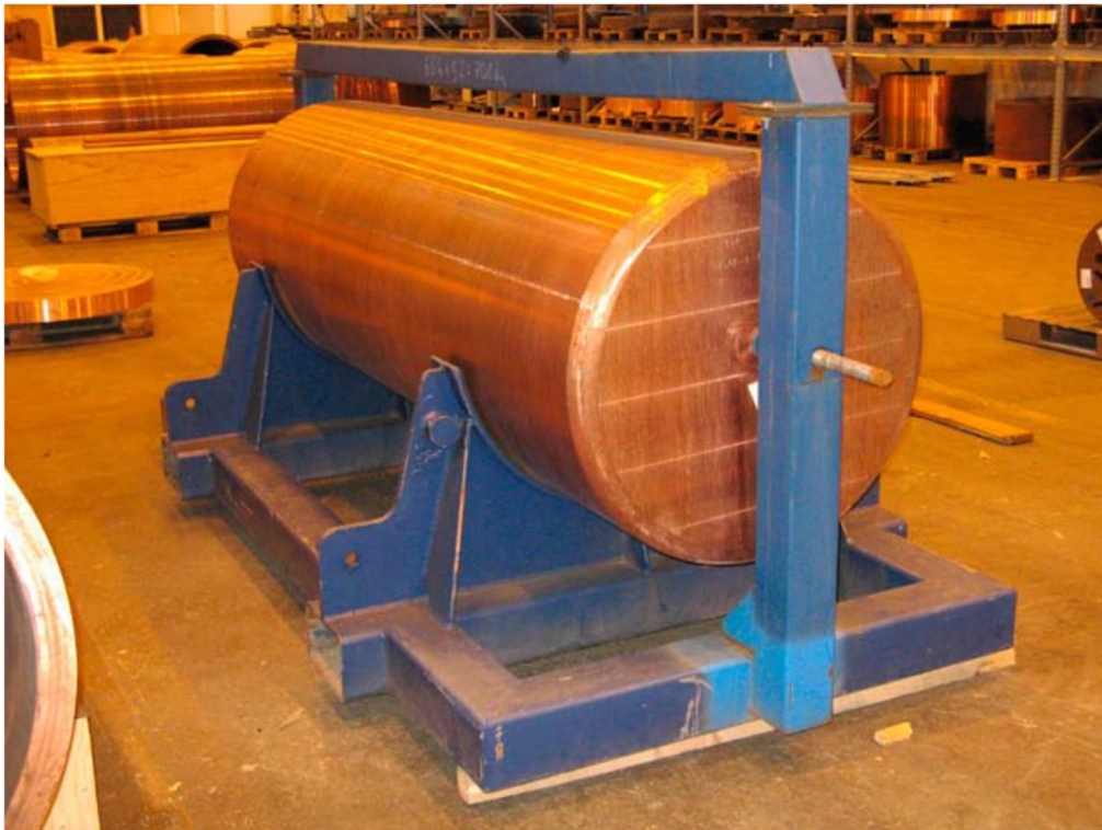
Figure 2-5: Large copper ingot for the production of copper tubes (SKB, 2010)
