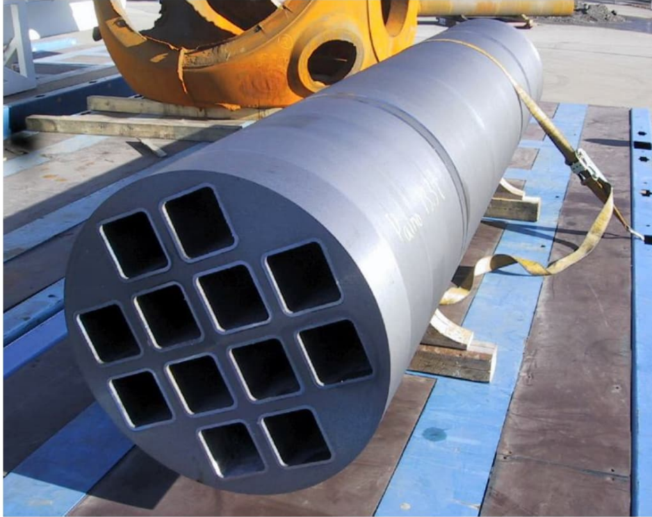
Figure 2-4: Machined insert for BWR spent fuel (Raiko, 2003)
