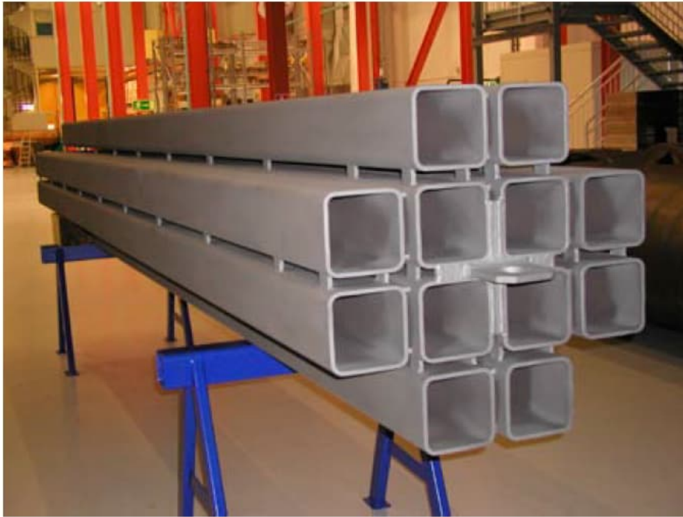
Figure 2-3: Steel tube cassette after manufacturing (SKB, 2010).
